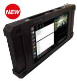
Enterpise is a unique hand held portable real time analyser of Streaming IP and ASI based services encoded as MPEG-2, H264 and others – with an intuitive graphical control interface. It's intended to cater for the huge increase in internet streaming traffic that needs a convenient compliance tool that can ensure services can be successfully decoded by consumers. It's a small, ruggedized, hand held portable tablet-like enclosure with a
